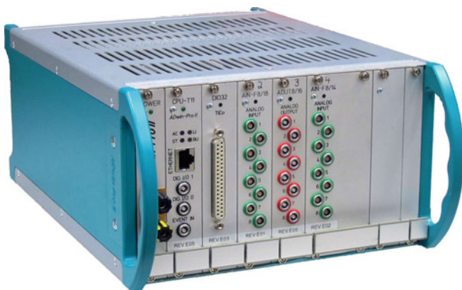
Fig. 4.22 Picture of the ADwin automat showing the front panel with an 18 an 14 bit analog input card an a 16 bit analog output card
