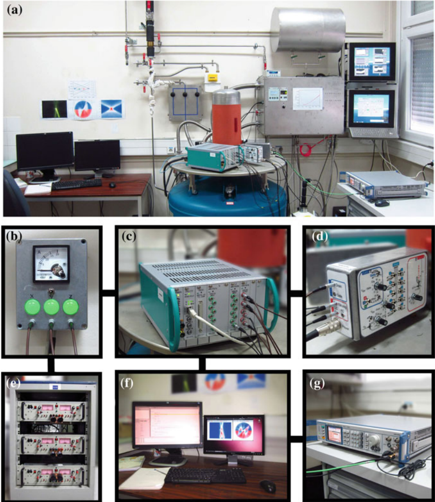
Fig. 4.2 a Picture of the experimental setup. The computer (f) controls the microwave source (g) and the ADwin real time data acquisition unit (c). The latter, in turn, operates the signal transducer (d) and the power supplies of the vector magnet, which are situated in the basement (e) via a remote terminal (b). The three LEDs in (b) indicate if the coils are operating. In case of a quench, the corresponding power supply is shut down automatically, and the LEDs will turn off. Further details of the individual parts of the experiment are explained in the text
